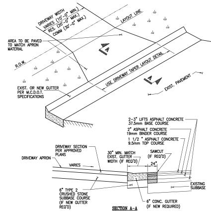
EXISTING PAVEMENT SHALL BE SAWCUT PRIOR TO GUTTER REPLACEMENT. ALL PAVEMENT JOINTS SHALL BE TACK COATED AND SEALED WITH BITUMINOUS SEALER.
